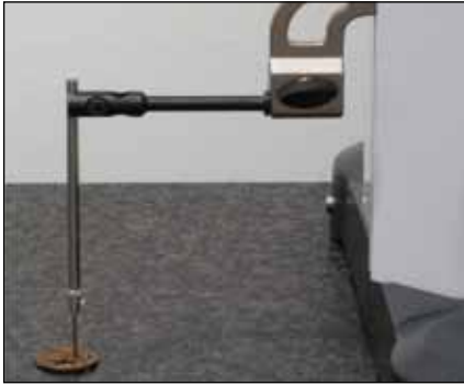
Height measurement of a small board (TA-IH-109/V-50.5/TA-MI-118)
