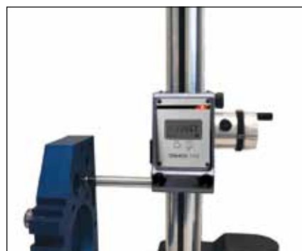
Measuring of centerline distances (TVM5)
