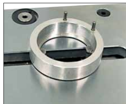
Checking of internal grooves (TELS10)
