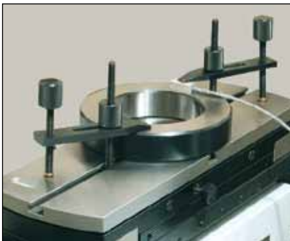
Integrated temperature compensation system TempComp
