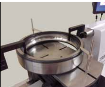
CNC controlled internal measurement of a bearing ring
