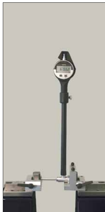
Setting of 2-point bore gauges (TEL5/TA-SU-301)
