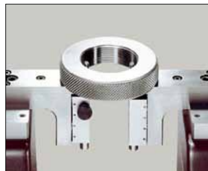
HPA: Checking of thread ring gauges (TEL18)
