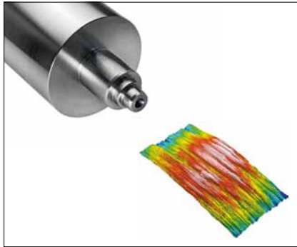
Steel Surface spinning measurement on a printing roll (DHM S2)
