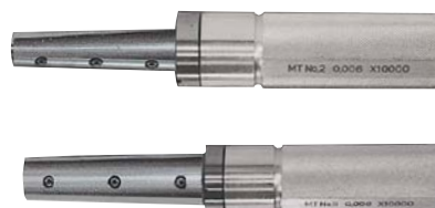
●内径モールステーパ3連式測定用 Three places measuring head for conicity measurement of Morse taper
