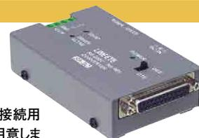
interface for connection with personal computer to change RS232C is available as option. DI-E2 can max.31units of DI-20 connect with one personal computer.
