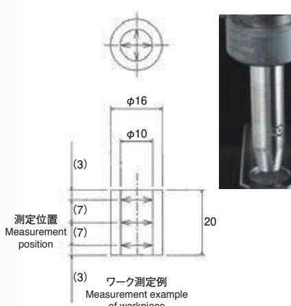
Measurement is made at six points in X-Y directions of the internal diameter of a workpiece by one measuring head, which is then transferred to the pass-fail screening lane. A ball screw is used for positioning of the measuring head and transferring the workpiece, and an air micrometer (single type) and a PLM are used for measurement and screening respectively.
