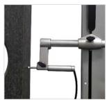
**Perpendicularity** Squareness measurements with electronic probe (V6)
