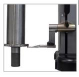
**Height Measurements** Height, thickness and chain of dimensions measurements
