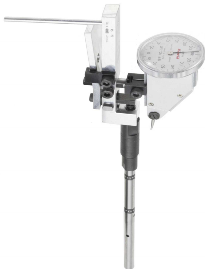
Valve Seat Face Runout Checker. 2 row type
