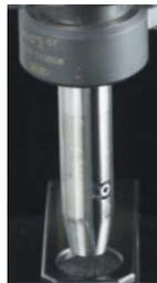
Measurement is made at six points in X-Y directions of the internal diameter of a workpiece by one measuring head, which is then transferred to the pass-fail screening lane. A ball screw is used for positioning of the measuring head and transferring the workpiece, and an air micrometer (single type) and a PLM are used for measurement and screening respectively.
