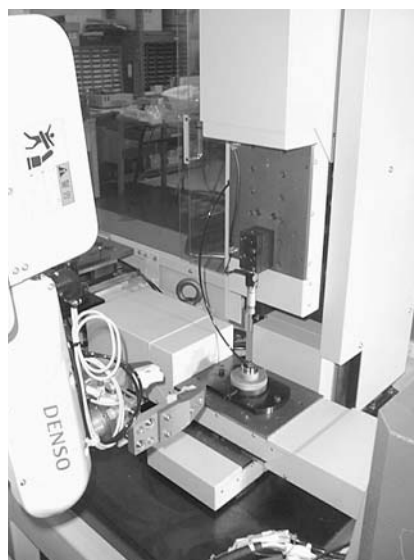
自社製精密テーブルで構築した三次元測定部 3D Coordinate measuring station by our original “High Accuracy Positioning Systems with BACK Lead Screws (PAT.)”
